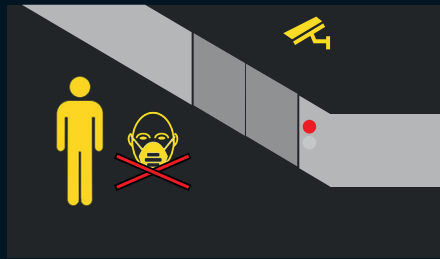
Scan of the person according to previously defined protective clothing characteristics (mask, gloves, suits etc.).
